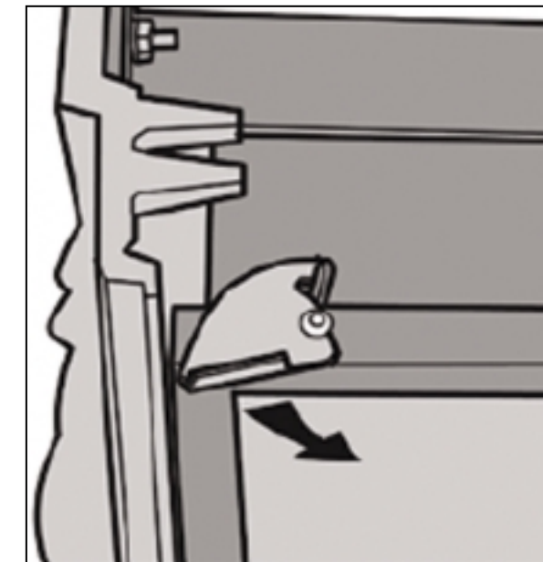
Fig 10. Swivel the latches to release the glass frame.
