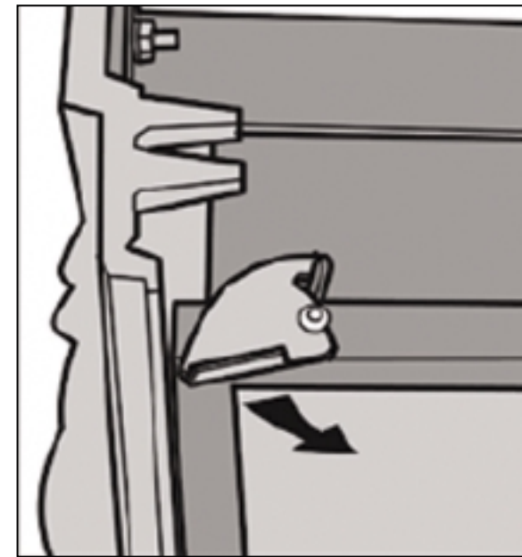
Fig 19. Remove the stove top and front, then swivel the latches to release the glass frame.
